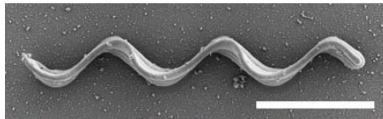
Figure 4: Hydrogel ABF in SEM top view; Scale bar: 10 \mu\text{m}
