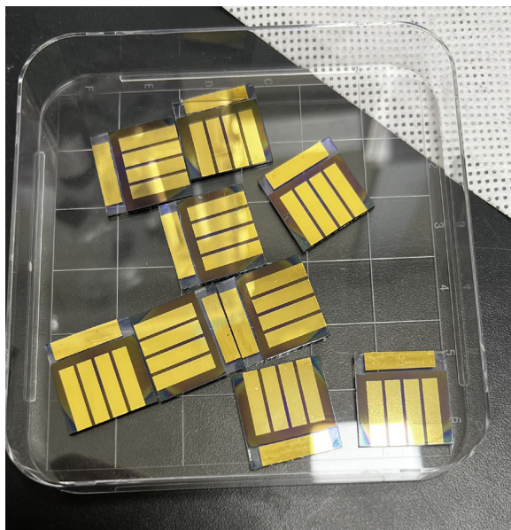
Perovskite solar cells fabricated in lab scale by the author.
